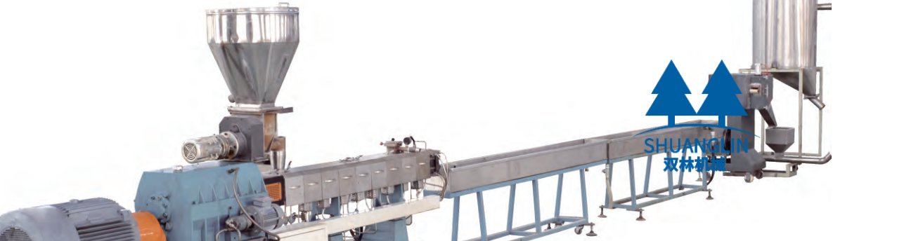
采用平行同向双螺杆挤出机 Parallel twin screw co-rotating extruder
